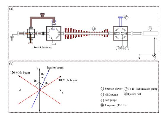
Figure 4.6: Orientation of optical dipole and barrier beam in the experimental setup: (a) Schematic: Side view of experimental setup [1]. (b) Schematic showing orientation of red detuned dipole beam and the blue detuned barrier beam with respect to imaging axis (y-direction). 110 MHz beam makes an angle  $\theta_1 \sim -25^\circ$  and 120 MHz beam makes an angle  $\theta_2 \sim 30^\circ$ . The optical barrier beam is oriented at  $\theta_3 \sim 10^\circ$ .
