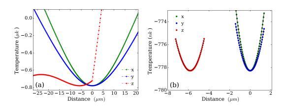
Figure 4.7: Modelling of the total trapping potential: (a) Cross sections along x, y, z direction of the numerically simulated trapping potential ( $U_{\text{Total}}$ ) across the trap minima at P = 3.6 mW. (b) Shows the second order polynomial fit (solid black lines) to the cross sections near the trap minima. from the fit, trap frequencies are extimated to be  $\nu_{\rm x} = 116$  Hz ,  $\nu_{\rm y} = 99$  Hz ,  $\nu_{\rm z} = 83$  Hz
