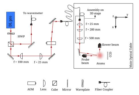
Figure 4.9: Optical layout for barrier beam preparation
