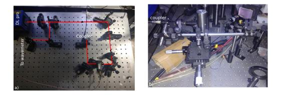
Figure 4.10: Image showing the setup to generate optical barrier: (a) Beam prepared on a separate optical table using a tunable DLpro laser diode. The output of this laser diode is split into two beams. one of the beams is transported to the main optical table and another beam is sent to wavemeter for monitoring the wavelength of the beam. (b) Shows the assembly of fiber coupler and three lenses, mounted on 3D stage to align the beam with respect to atomic cloud
