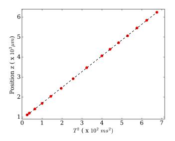
Figure 4.4: Magnification of the imaging system: Plot shows the center position of an atomic cloud falling freely under gravity. Dashed black line shows the linear fit to data. From the slope of the straight line, magnification of our imaging system is estimated as 1.61
