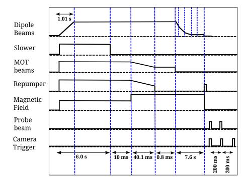
Figure 4.2: Experimental sequence: Plot shows the ON and OFF time for different optical and magnetic fields. First, two of the three camera trigger pulses overlap with two probe laser pulses with a wait time of 200 ms between them which depicts the detection scheme.
