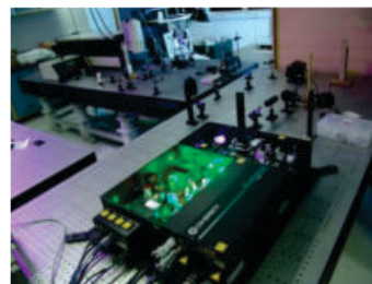
Top: Structure of human HGPRT with bound substrate (guanine monophosphate (1HMP)). Bottom: Raman Lab showing the Ti-S based tunable deep UV excitation source.
