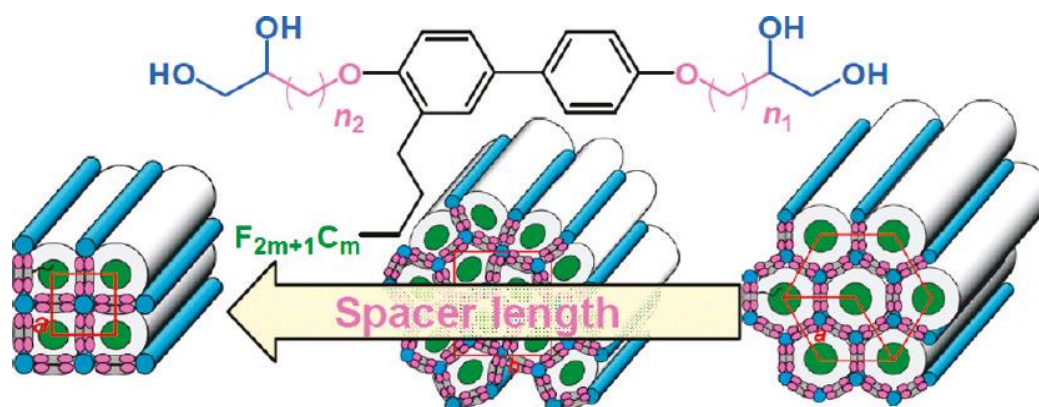
Figure 4.1. Liquid-crystalline honeycomb structures composed of cylinders having hexagonal, pentagonal, and square cross section. (Adopted from Xiaohong et al. J. Am. Chem. Soc. 2011 , 133, 7872–7881).
