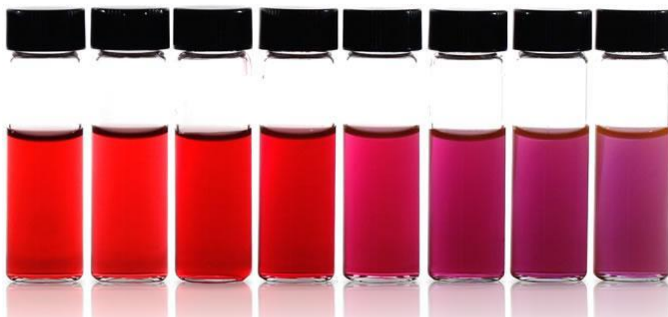
Figure 1.1 Gold nanoparticles of different sizes showing variation in the plasmon color (adapted from reference 5).
