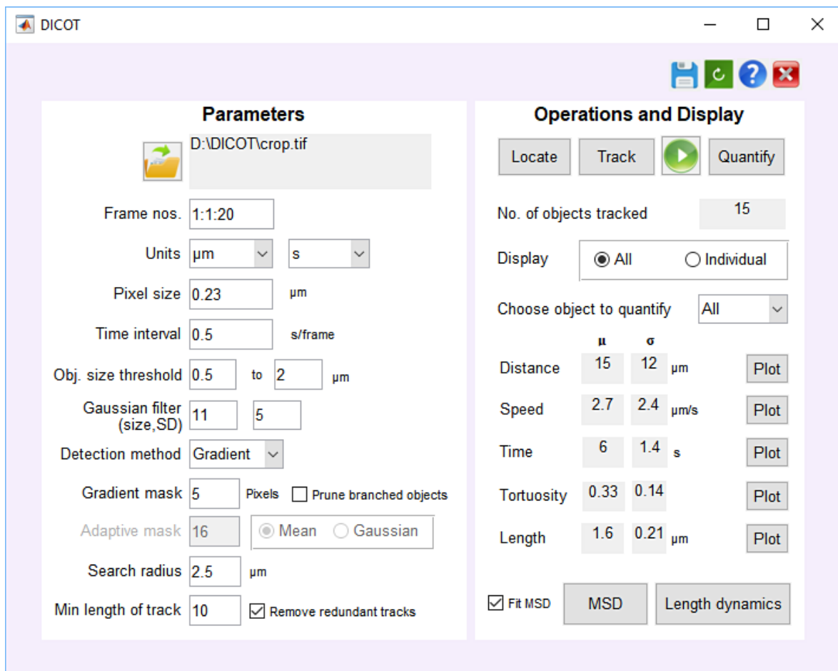
Figure 5.2. DICOT interface. The GUI allows the user to provide input in the ‘Parameters’ panel, which is processed to obtain statistics that are displayed in the ‘Operations and Display’ panel.
