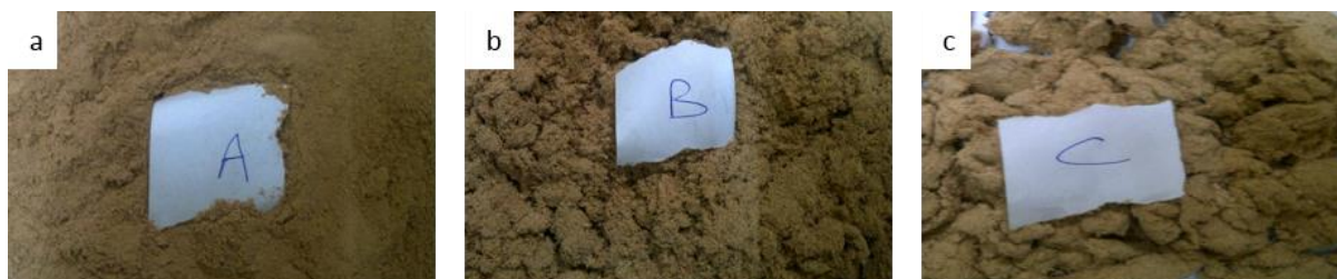
Figure 4: Photographs of leather buffing dust (a) from leather board, (b) from an intermediate step of leather sole manufacturing process, (c) from the final step of leather sole manufacturing process
