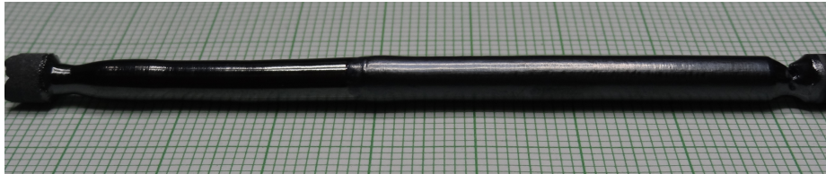
Figure 3.10: The grown crystal boule of Ba_2Fe_2O_5 (experiment 2)
