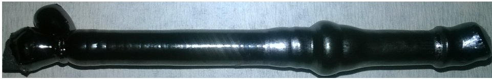
Figure 3.9: The grown crystal boule of Ba_2Fe_2O_5 (experiment 1)
