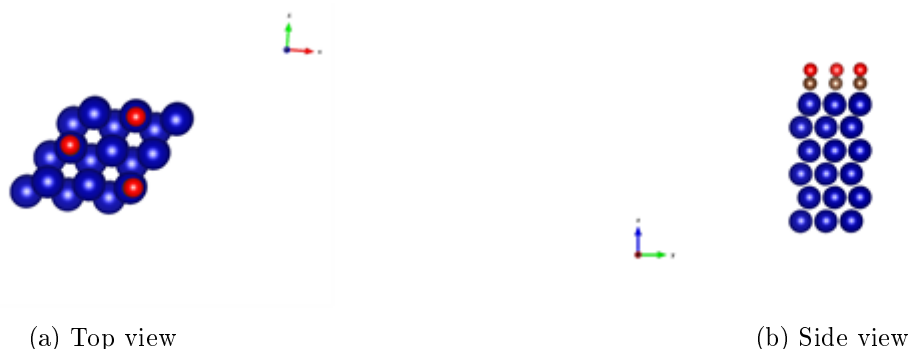
Figure 3.7: (\sqrt{3} \times \sqrt{3})R30^\circ adsorbate coverage for CO at \theta = 1/3 on a p(3x3), 6-layered Co Vacuum slab
