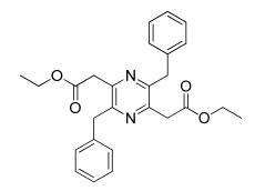
**Yield** = 65 % **UV** ( $\lambda_{max}$ ) = 204 nm, 281 nm; **Fluoroscence** ( $\lambda_{ex}$ ) = 281 nm, ( $\lambda_{em}$ ) = 443 nm; <sup>1</sup>**H NMR** (400 MHz, CDCl<sub>3</sub>)  $\delta$  7.27–7.14 (m, 10H), 4.18 (s, 4H), 4.07 (q, *J* = 7.1 Hz, 4H), 3.81 (s, 4H), 1.19 (t, *J* = 7.1 Hz, 6H).
