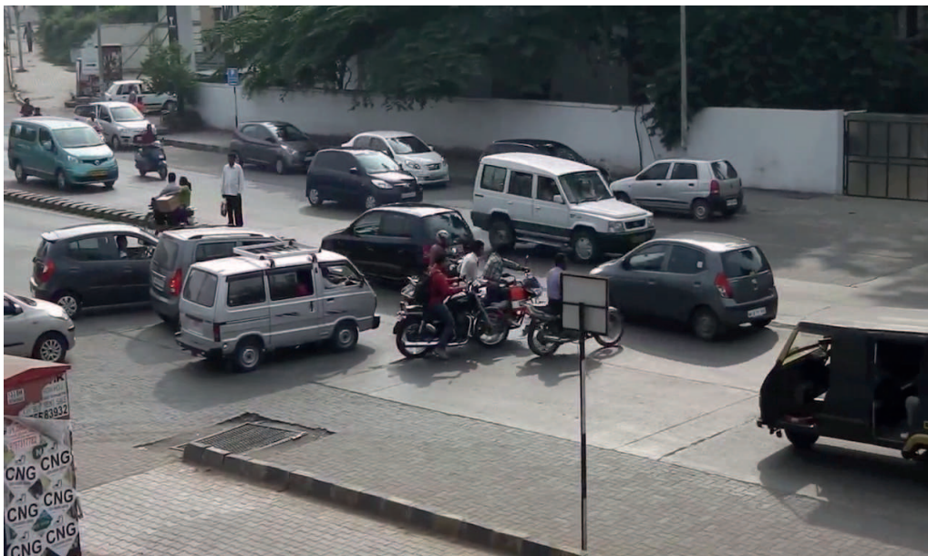
Figure 5.3: This image shows a bunch of vehicles from the cross lane crossing the intersection as a 'herd'. Since it is not very easy for a single vehicle to cross a crowded road intersection.
