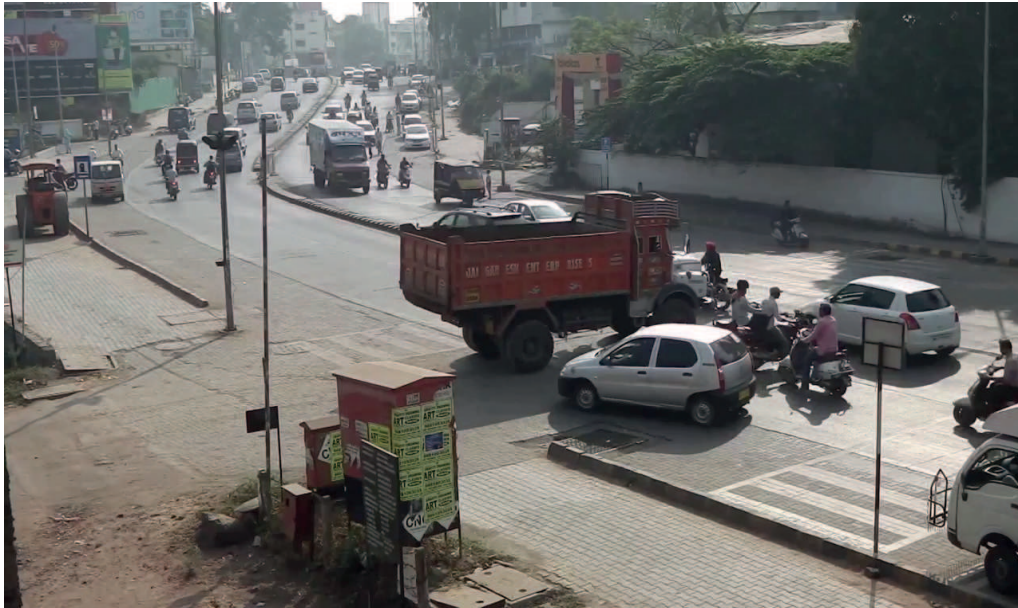
Figure 5.1: The red truck is an example of how a bigger vehicle can encroach its way through the main lane to get across.
