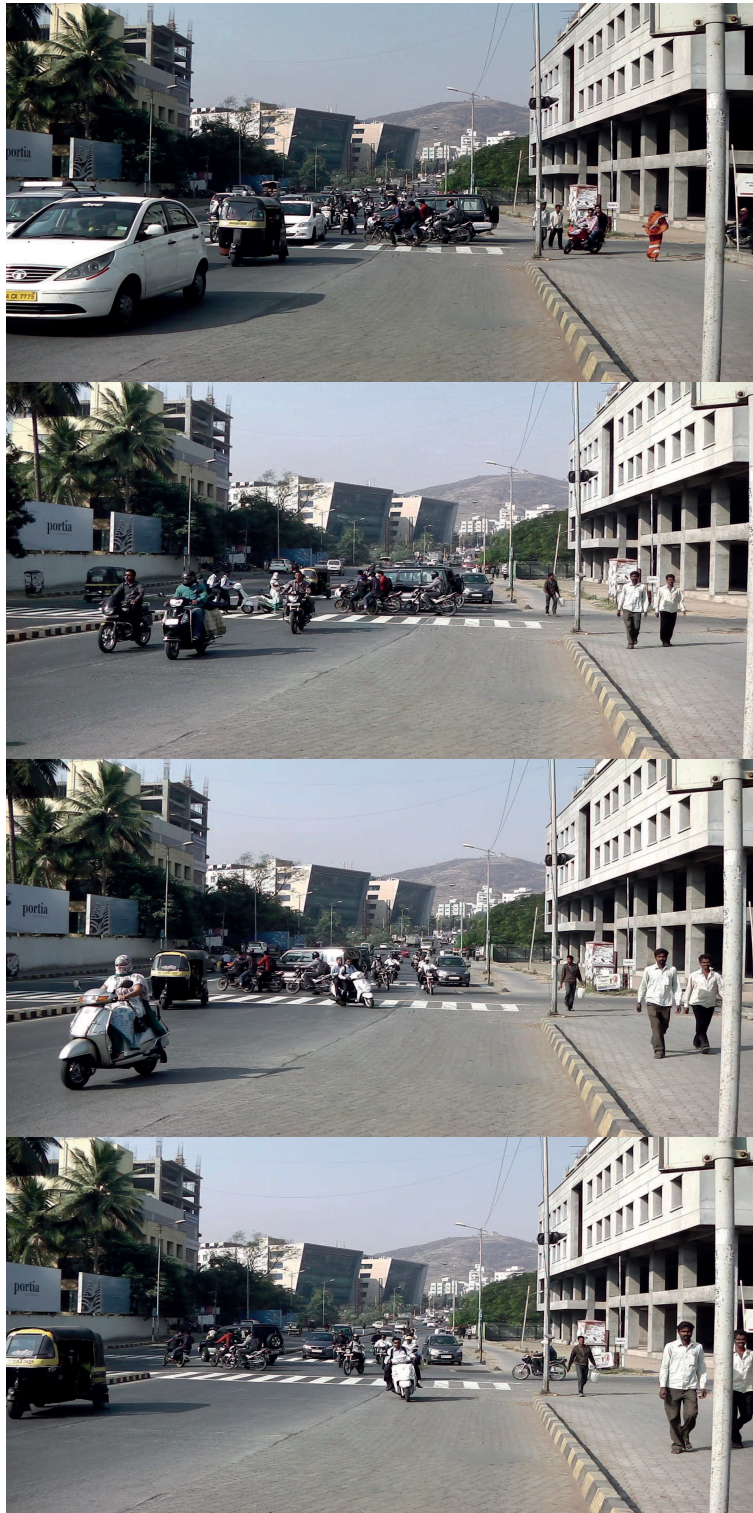
Figure 5.5: The four images are continuous clicks of a bunch of vehicles from the cross lane trying to cross through the main lane. The first image shows how vehicles are accumulating to form a 'herd'. In the second image, the herd encroaches into the first row of vehicles of the main lane. The third image shows the herd encroaching into the second row of vehicles in the main lane. In the last image, they are out of the intersection.
