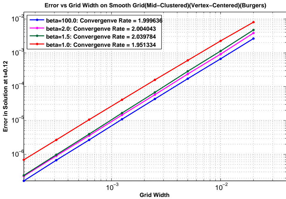
Figure 3.14: Convergence Analysis on Smooth Grid in which cells are clustered at the middle: beta = 1.0 results in slow convergence
