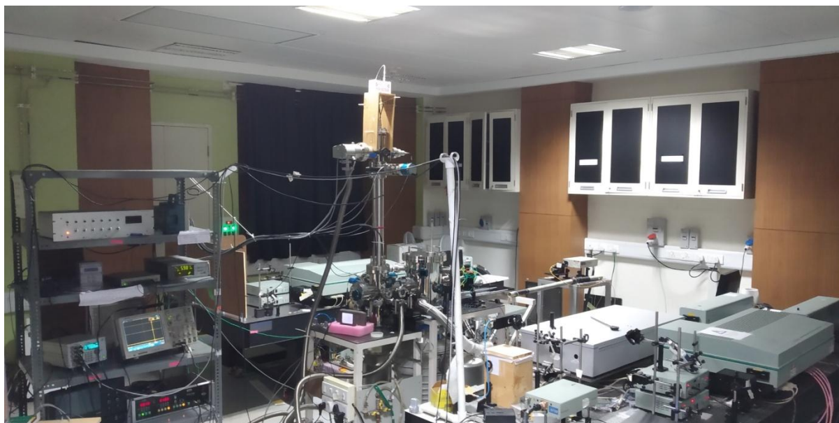
Figure 2.7: Laboratory photograph showing home built jet cooled TOF-MS.
