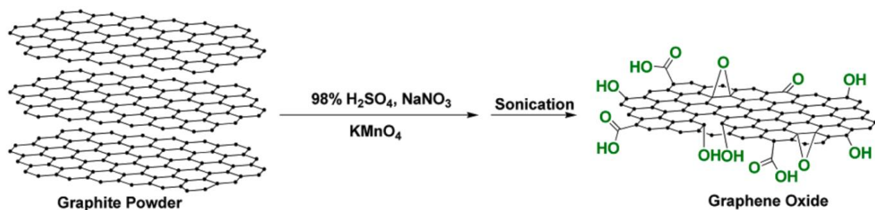
Figure 1.8: Synthesis of graphene oxide (GO) from graphene by modified Hummers method (adapted from Xu et al. ACS Appl. Mater. Interfaces 2014, 6, 17265-17276).
