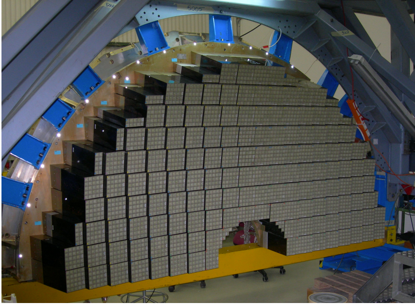
FIGURE 3.8: One “D” formed out of supercrystals which makes half of each ECal endcap
