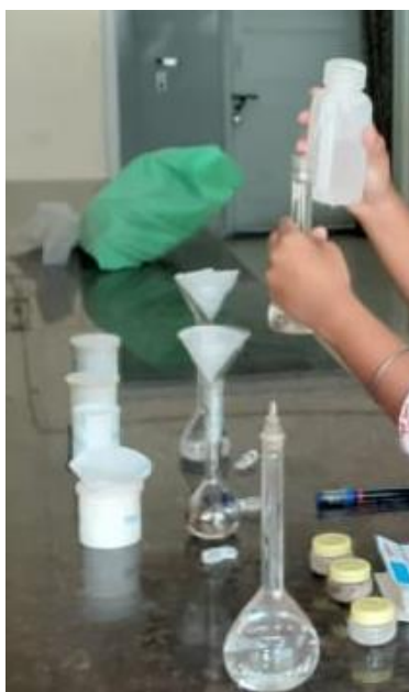
Fig 2.5: The above image shows filtering of dissolved rock samples for ICPMS analysis
