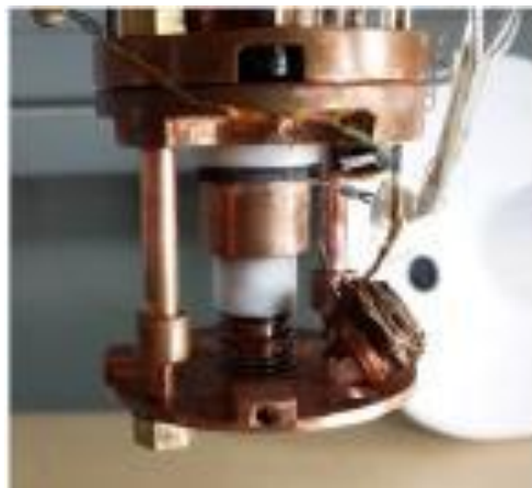
Figure 5.2 Spring-loaded sample holder attached to the cold head of CCR.
