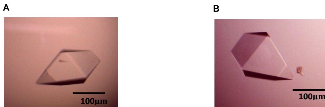
Figure 5.3. Crystals obtained after optimization of initial condition. (A) Single crystals obtained in condition 1. (B) Single crystals obtained in condition 2. Morphologically the crystals look identical to each other, however crystals in condition 1 belong to tetragonal space group and diffracted poorly. The crystals in condition 2 belong to orthorhombic space group and diffracted better.
