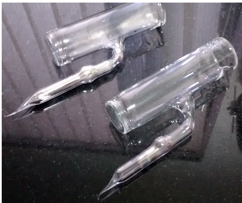
Figure 4.1: First pair of Rubidium vapour cells fabricated at IISER Pune
