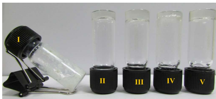
Figure 4.3: (I) Solubility of peptide P1 (10 mg/mL) in 1× PBS. Formation of organogel (10 mg/mL) of peptide P1 in different aromatic solvent (II) Benzene (III) Toluene (IV) Xylene (V) Mesitylene.
