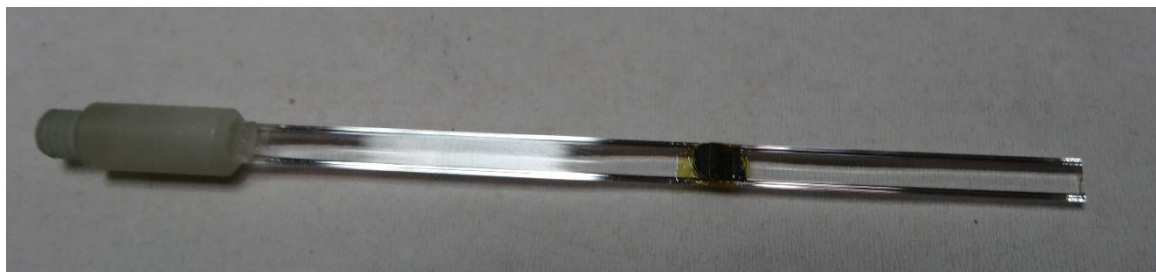
Fig 2.6 One of the sample pellets glued to the quartz sample holder for VSM measurements
