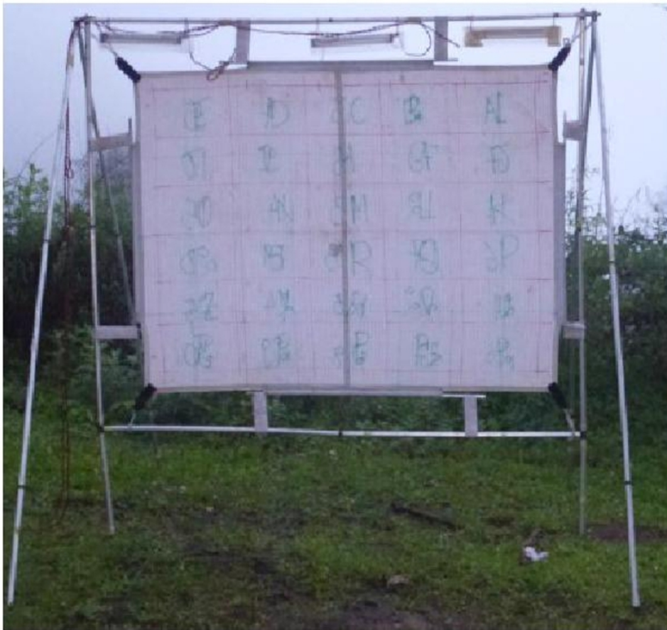
Figure 2.4 Portable moth-screen, consisting of a light-weight hollow aluminium pipes connected via screws and bolts into a frame. 2-UV (8W each) and 1 white light (8W) actinic tubes were used to attract moths. Moths typically settled on the gridded cloth screen (160 cm X 110 cm).
