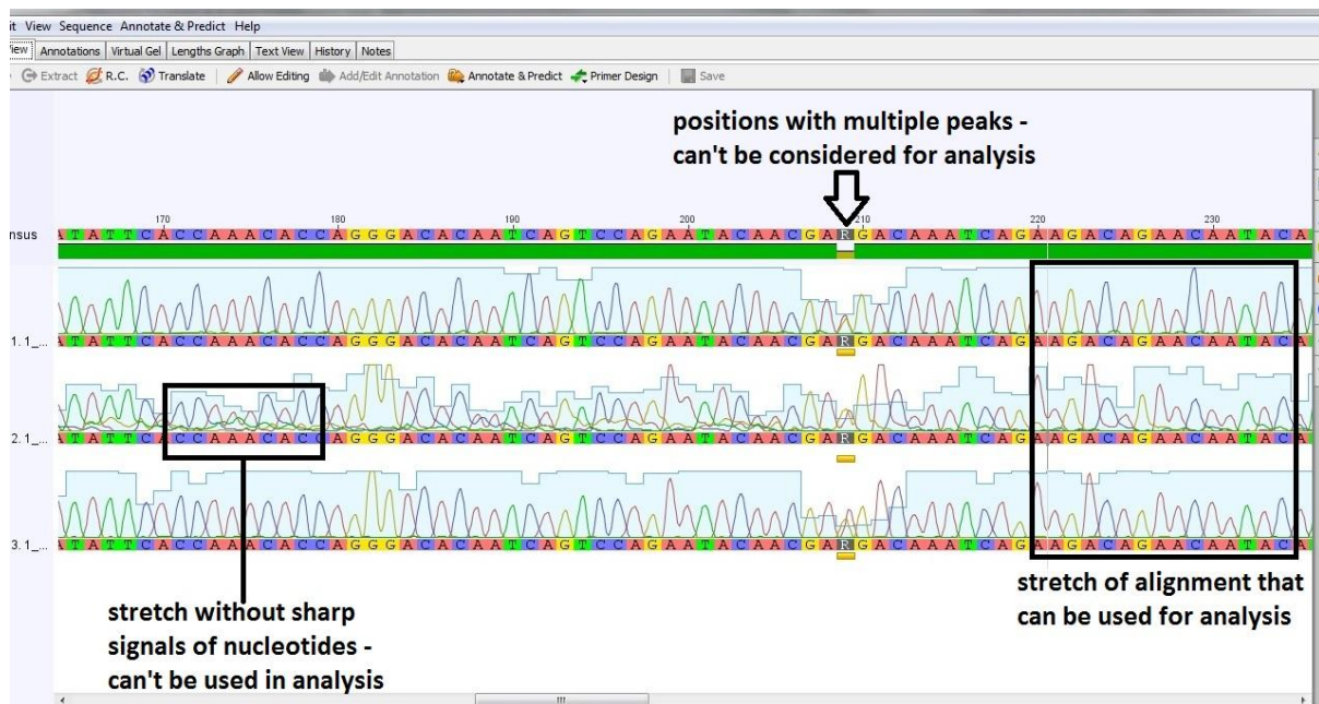
Figure B1: Geneious view showing regions in the alignment that can be selected for analysis based on the chromatograms
