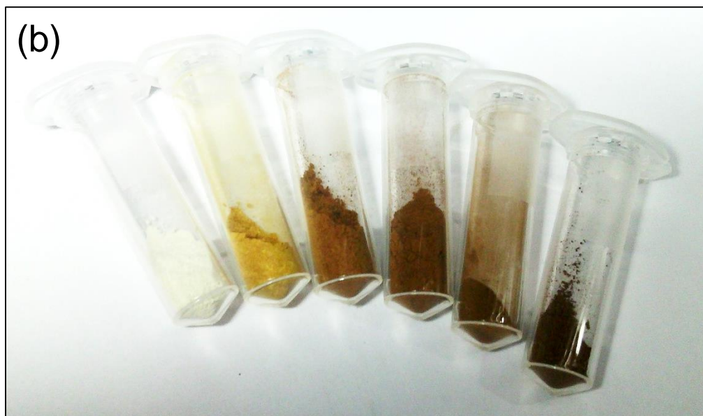
Fig. 4.2. (a) Tauc Plot of Zn 1-x Cd x O samples, (b) Color of the Zn 1-x Cd x O samples, from left x= 0, 0.2, 0.4, 0.6, 0.8, 1 .
