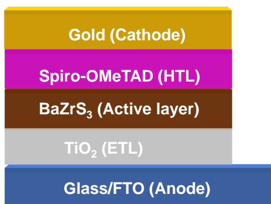
Figure 5.17: Planar architecture of fabricated solar cell device with layers from bottom to top as: FTO/ TiO 2 / BaZrS 3 NCs/ Spiro-MeOTAD/ Au.
