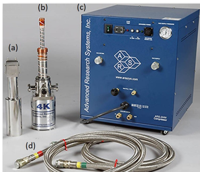
Figure 2.1: (a) vacuum shroud, (b) refrigerator, (c) compressor, and (d) Helium hoses are depicted.
