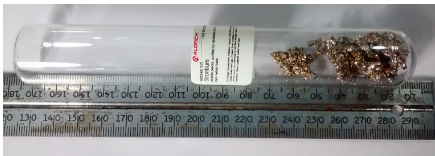
Figure 3.13: Strontium ampule: The ampule is broken inside a glove box and dendrite pieces are filled in the oven reservoir shown in Fig. 3.2(b).
