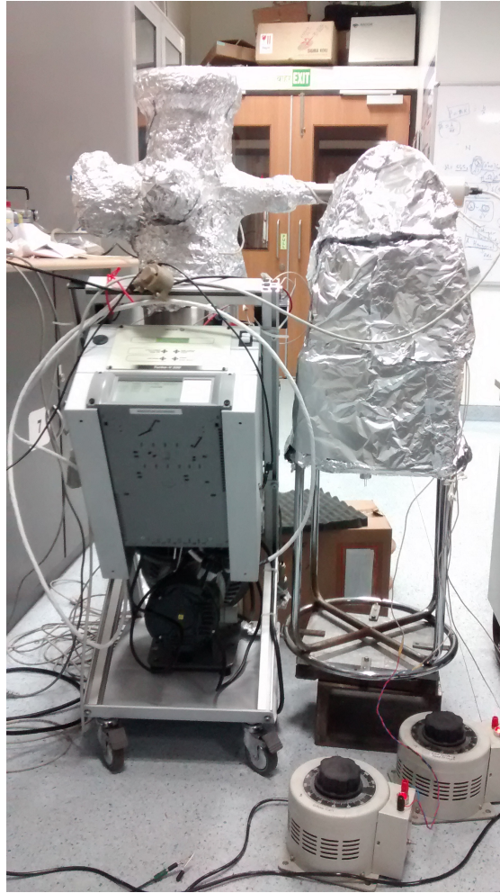
Figure 4.19: Baking of spectroscopy cell: A cage-like enclosure is used for baking. A heating coils are wrapped around the enclosure. The cell is baked by the convective and radiative heating mechanism.
