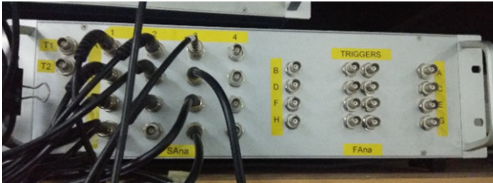
Figure 4.33: Analog voltage generator: Front panel of the FPGA based analog voltage generator.
