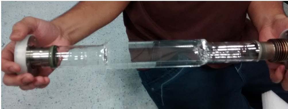
Figure 3.12: Quartz cell: The quartz cell provides the optical access for cooling and trapping laser beams.
