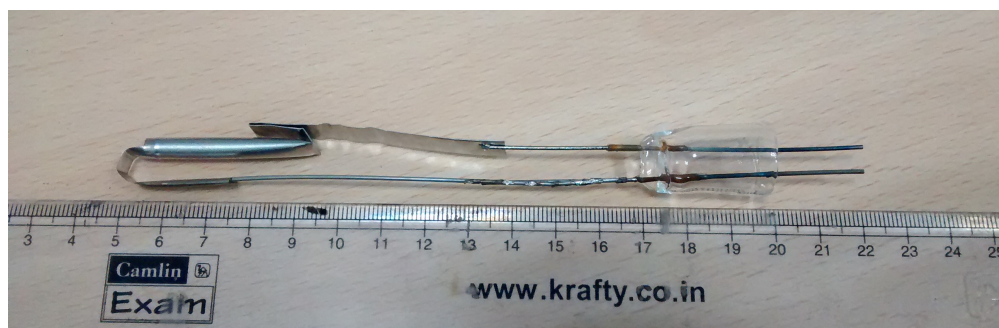
Figure 4.18: Sr dispenser: Sr dispenser is spot welded to the tungsten electrode. These electrodes provide the electrical connections for dispenser operation.
