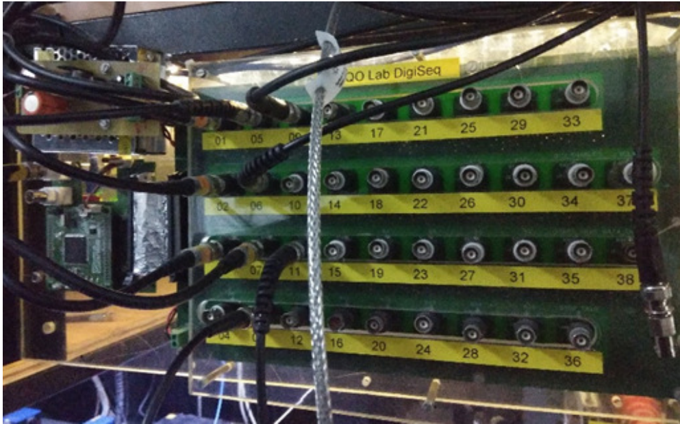
Figure 4.32: Digital sequencer: Front panel of the digital sequencer used for the generation of TTL pulses for the experiment.
