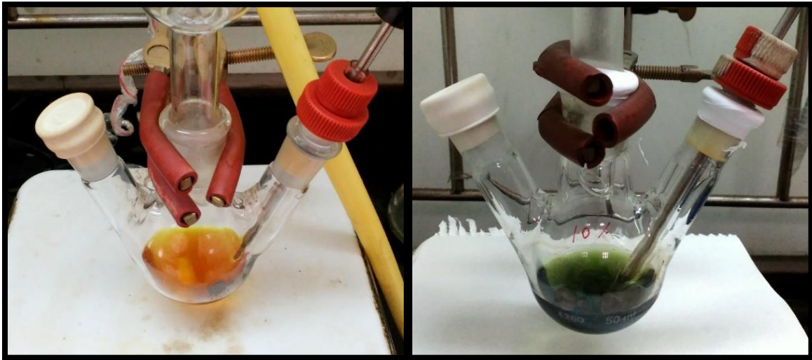
Figure 3: Photograph of the reaction mixture of the colloidal NCs a) 10% Mn doped \text{In}_2\text{O}_3 NCs showing reddish color, b) 10% Cr-10% Sn codoped \text{In}_2\text{O}_3 NCs showing intense bluish green color.
