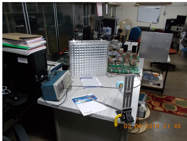
Figure 4.12: Experimental setup for the new method. The small disk on the stand is the Cd source. Behind each vertical array of squares, anode wire runs through the centre. As only six wires were used, the source has offset compared to the centre of detector.
