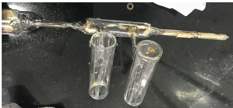
Figure 3.4: Cesium glass manifold. Cesium can be seen as golden coloured liquid spread through out the manifold.
