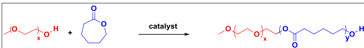
Figure 1.4 General Scheme for Ring Opening Polymerization (ROP)
