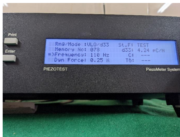
Figure 4A.20: Photograph of the piezometer displaying the d_{33} value obtained on an of unpoled 20 wt% MTPBB/PDMS film.
