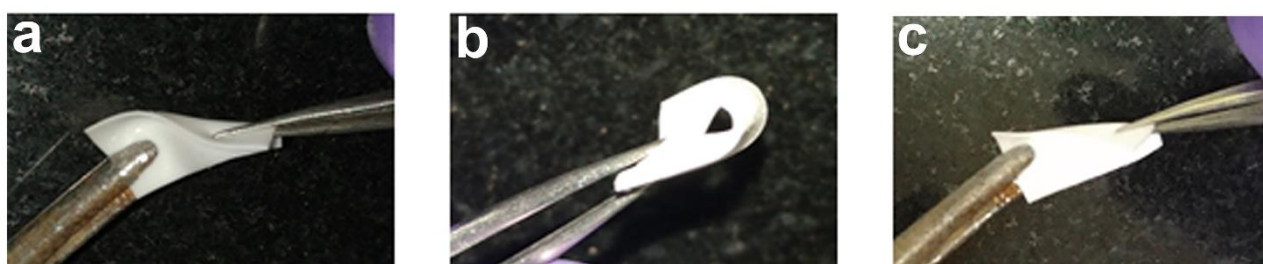
Figure 3A.16: Flexible composites exhibiting (a) bending (b) rolling and (c) stretching operations.
