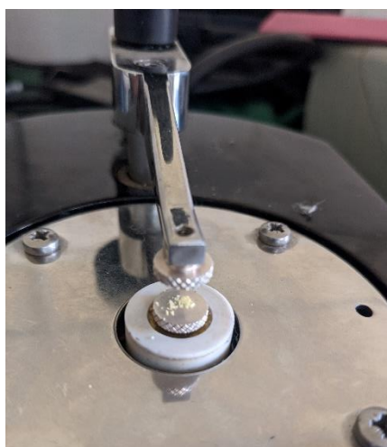
Figure 4A.16: Photograph of the broken crystal while performing d_{33} measurements on piezometer
