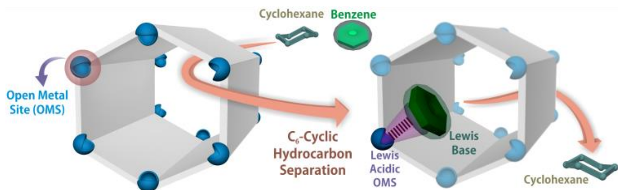
Scheme 3B.1. Schematic representation of the pursued strategy: exploiting Lewis acidic coordinatively unsaturated sites of an OMS-rich MOF platform, to exhibit selective interplay with aromatic, planar Lewis base benzene over its aliphatic, non-planar C 6 -analogue cyclohexane.
