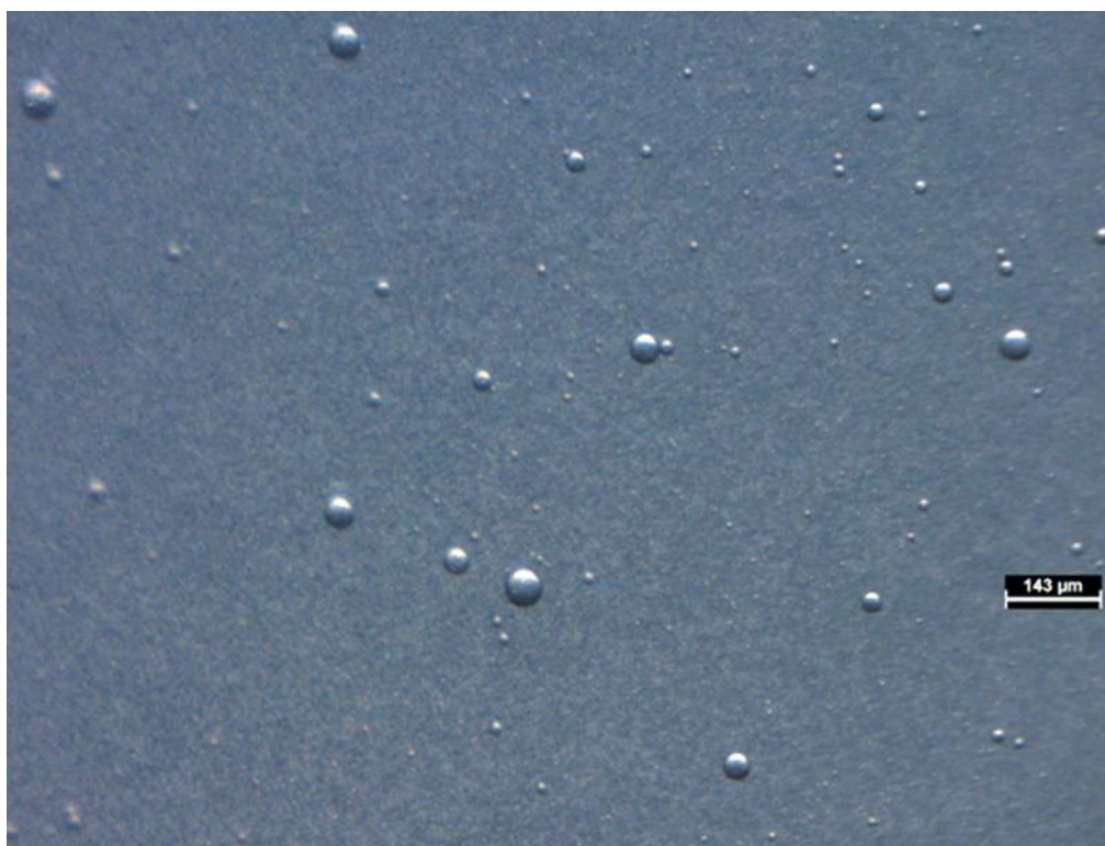
Appendix 4.27. Optical microscope image of emulsion droplets, the approximate droplets size was found in micro metre scale.
