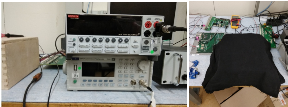
FIGURE 5.5: Setup for IV characterization. Image on the left shows front panel of Keithley Source-meter 2410 (instrument on top). Right image shows the module covered with a wooden box and black cloth.
