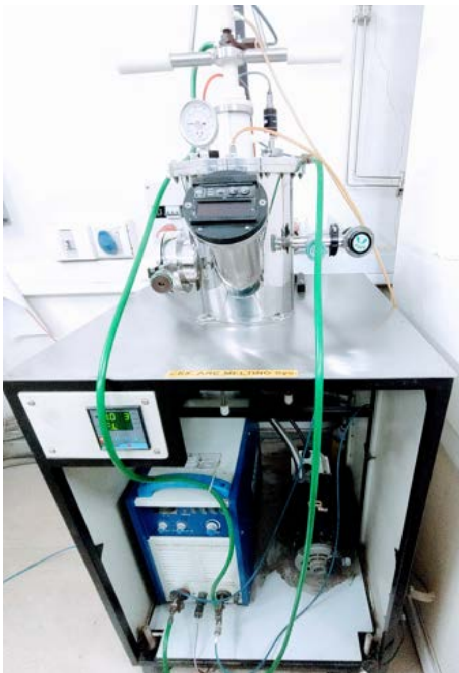
Figure 2.1: Arc melting machine with current source and vacuum pump
