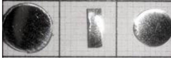
Figure 2.5: Sintered pellets of \text{Nb}_{0.83}\text{CoSb} for thermal and charge transport measurement in shape of disc and bar.
