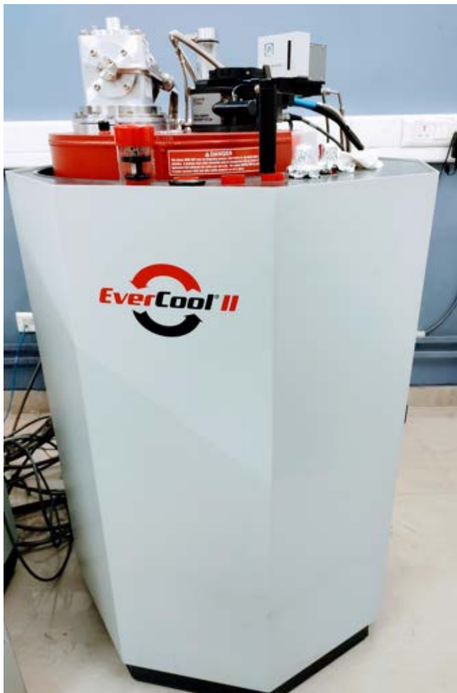
Figure 2.14: PPMS from Quantum Design in Lab 210 at IISER Pune.
