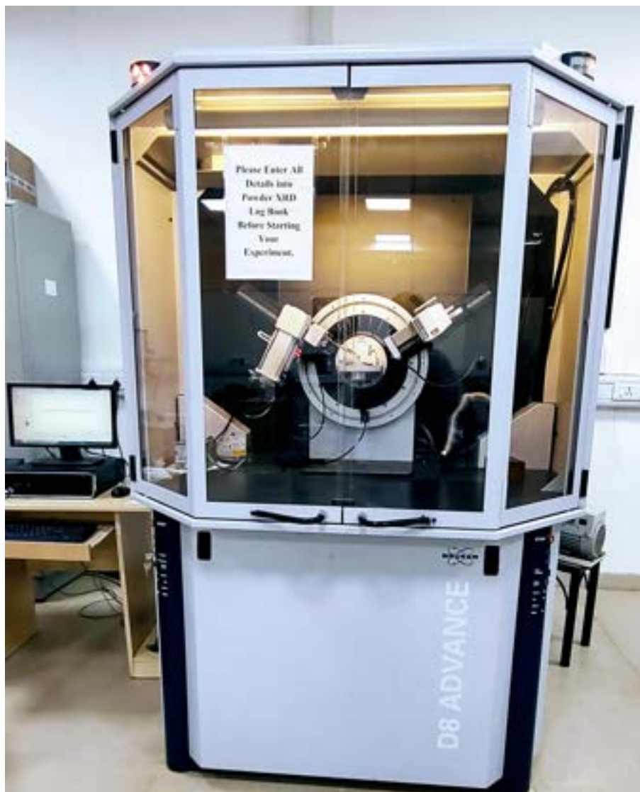
Figure 2.6: X-ray diffraction instrument Bruker, D8 Advance diffractometer at IISER Pune.
