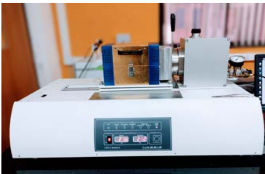
Figure 2.18: Linseis LSR-3, Germany for resistivity and Seebeck coefficient simultaneous measurements.
