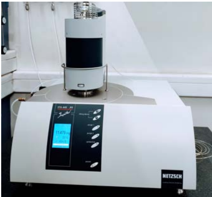
Figure 2.12: TGA/DSC From Netzsch, Germany for thermal analysis of sample.
