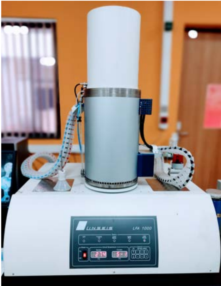
Figure 2.21: Laser Flash Analyzer (LFA) Linseis, Germany for thermal diffusivity measurements on disc shaped samples.
