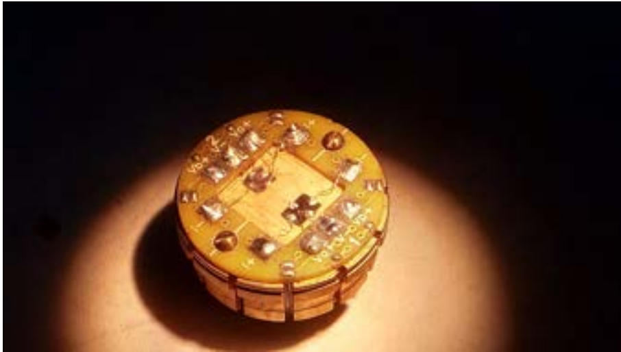
Figure 2.15: Hall puck for Hall measurement with two samples loaded for measurement in four probe geometry.
