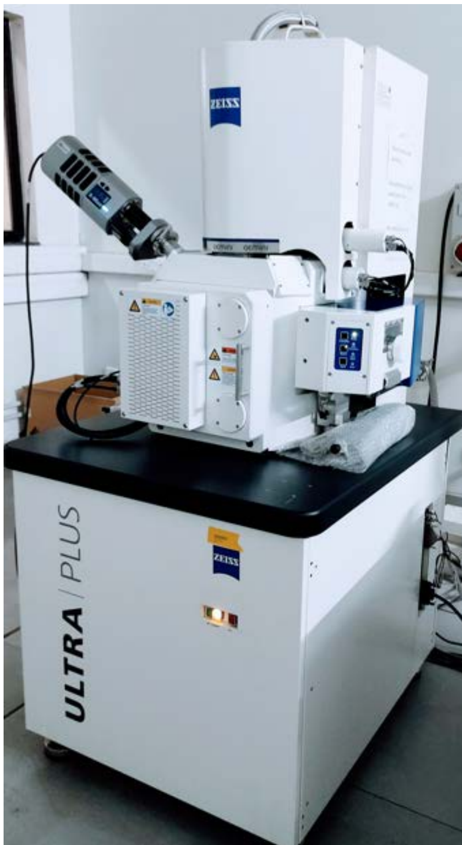
Figure 2.8: FESEM Ultra Zeiss plus at IISER Pune. The instrument was used for observing microstructure, chemical composition and EDX analysis.
