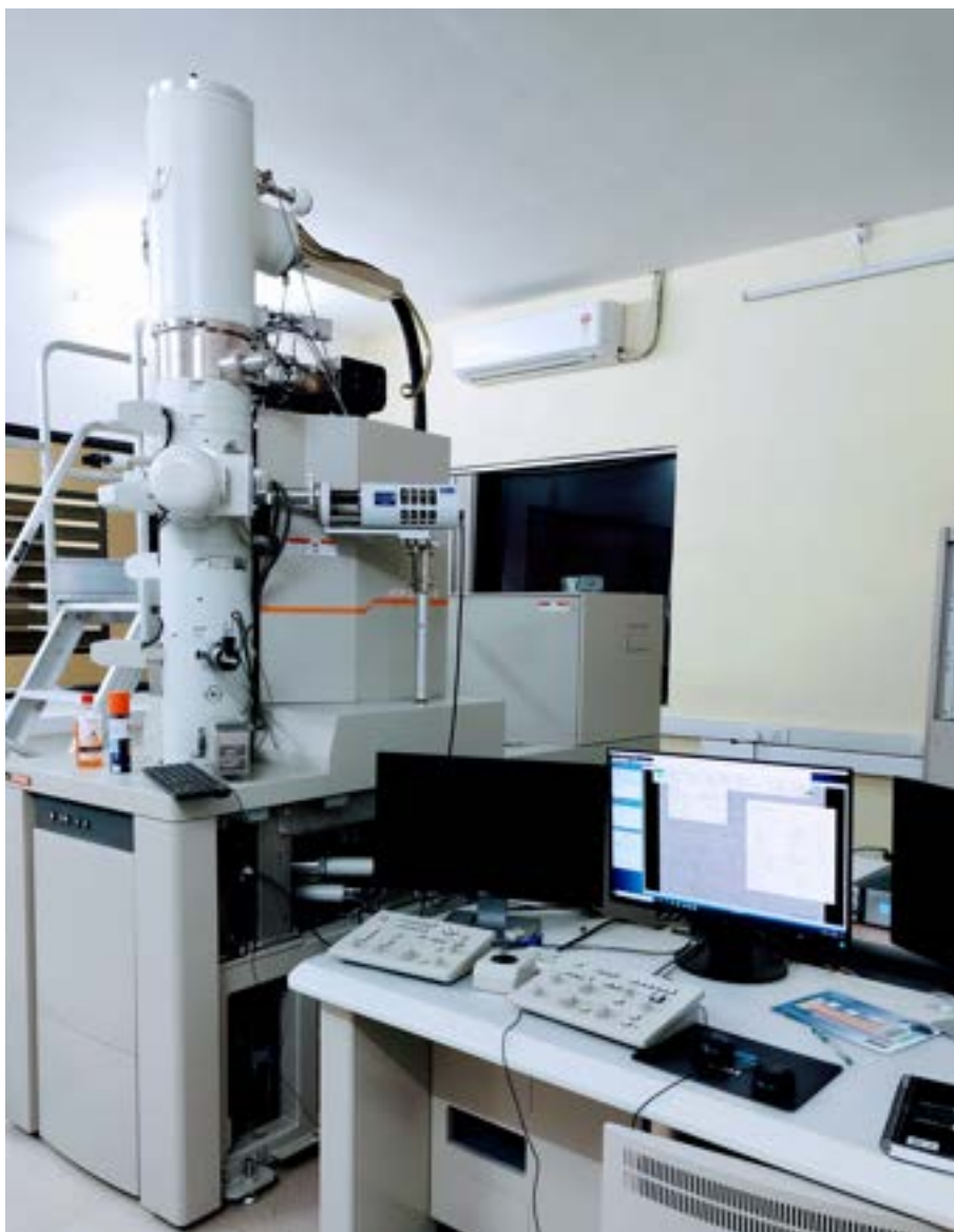
Figure 2.10: HRTEM JEOL JEM 2200FS at IISER Pune. The instrument was used for observing microstructure, selected area diffraction pattern (SAED), EDX analysis and chemical mapping.
