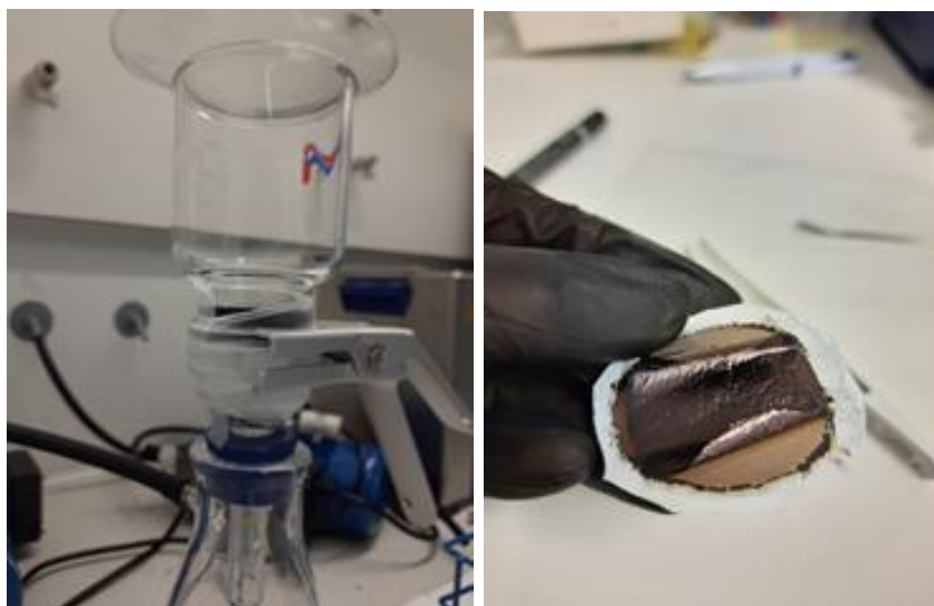
Figure 6: (a) Vacuum filtration setup, (b) Filtered freestanding V_2C film
