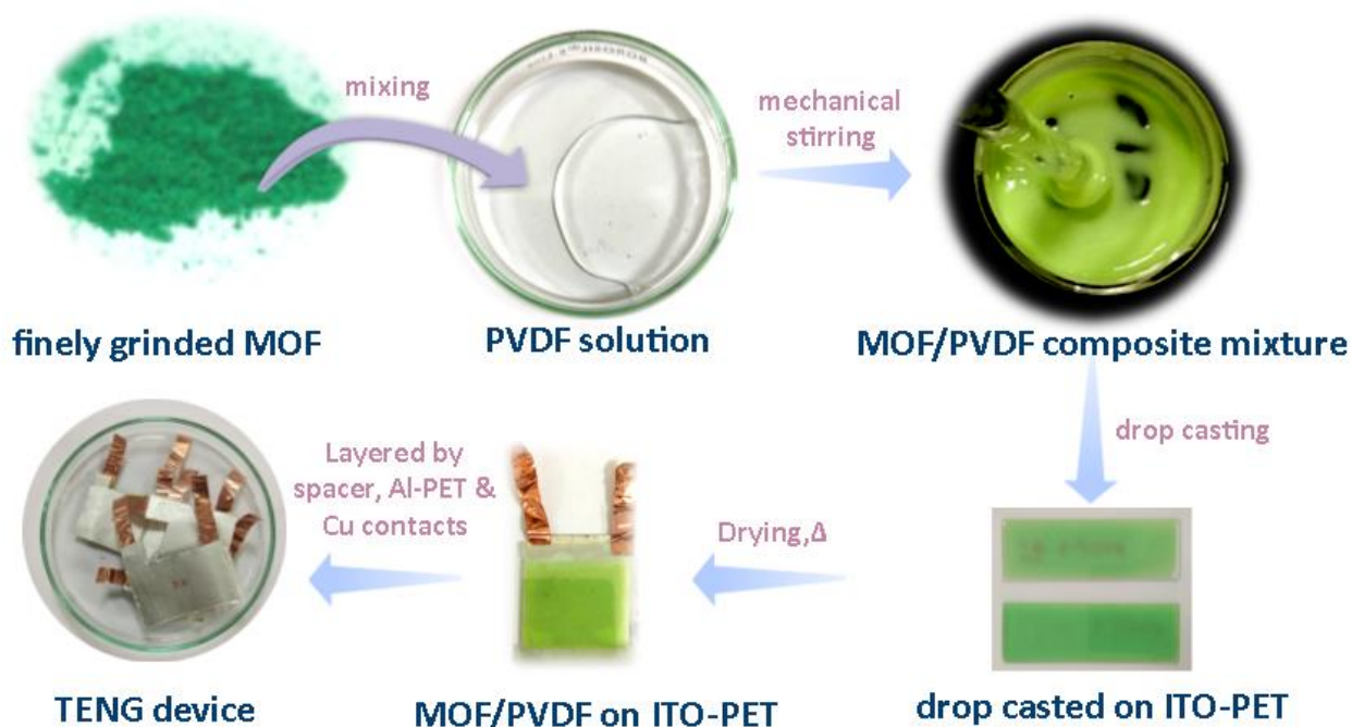
Scheme 1. A depiction of the sequential fabrication approach deployed for the IPMOP-n/PVDF composite-based mechanical energy harvesting device.
