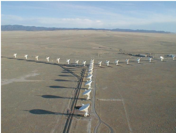
Figure 1.7: The ‘Wye’ of the Very Large Array(VLA) at New Mexico with 27 dishes making an effective dish of 4 km in diameter at its widest configuration *Image Credit: NRAO/AUI/NSF*
