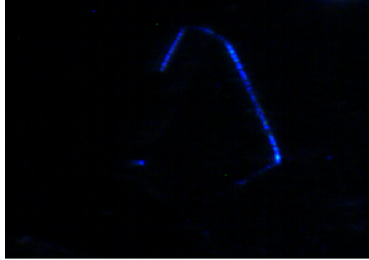
Figure 4.2: Dark field image of MoS_2 flake
