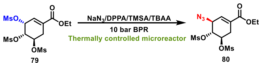
Scheme 3.1.3: Literature precedents of azidation under continuous flow
