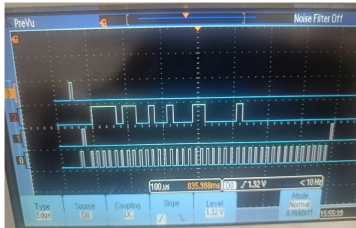
Figure 4.2- The representation of the frequency tuning word for the AD9850 for 1 MHz. Here 0 is for the W_CLK (reference clock), 1 is for CS (chip select) or FQ_UD, 2 is for DATA and 3 is for RESET.
