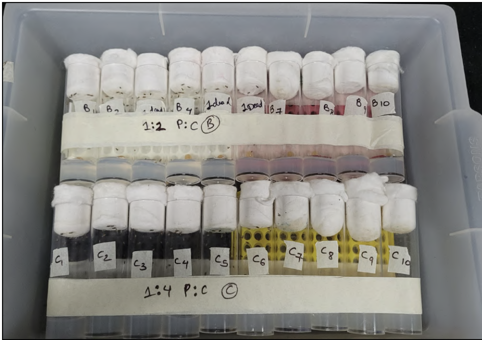
Image 2.4.3: Picture depicting the 10 serially labeled DIET vials for each of the containing 1:2 and 1:4 P:C food cups respectively at a measured distance of exactly 1 mm from the agar beds with an elevated surface and 100 ml RO water beneath.
