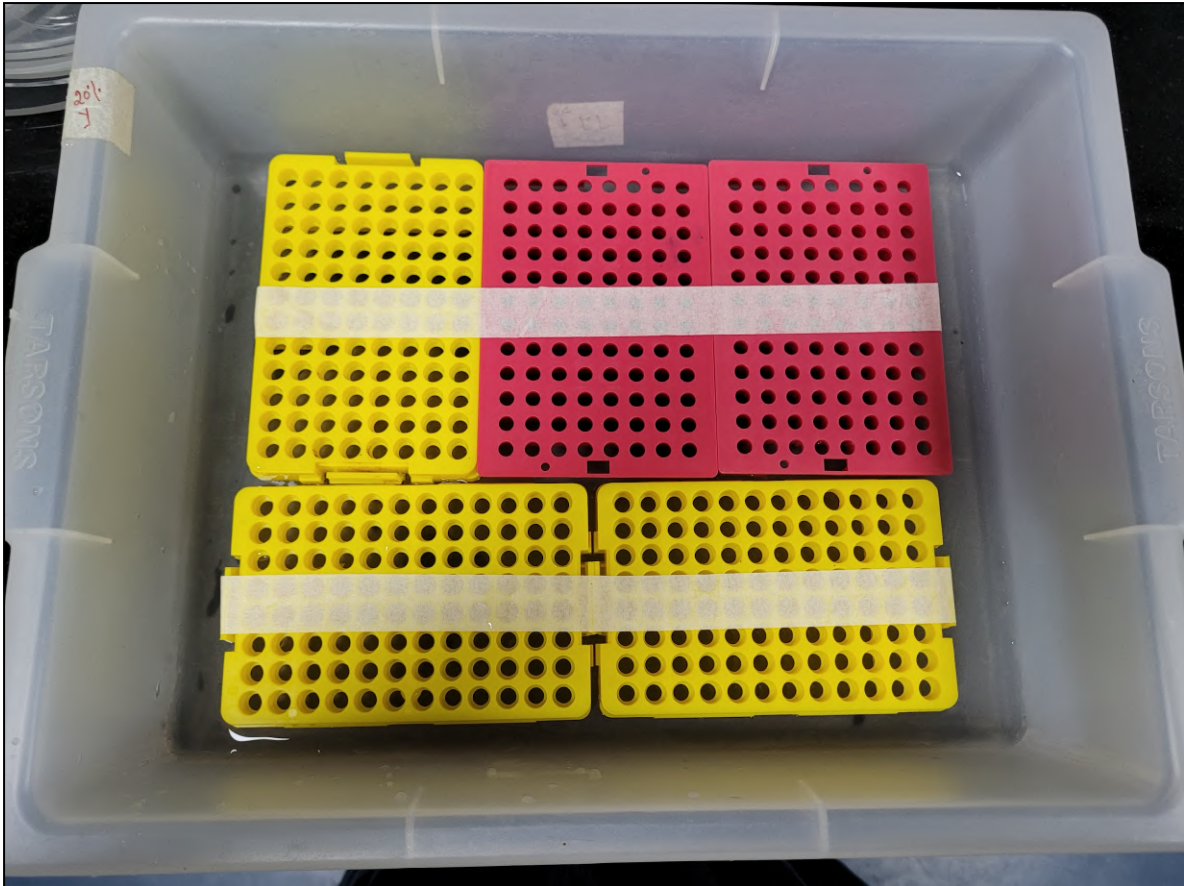
Image 2.4.1: Picture depicting the elevated surface made out of pipette tip box stages with 100 ml RO water beneath to reduce the evaporation such that the DIET vials do not get wet but have the humidity maintained through the big holes present in these stages
