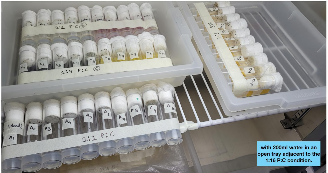
Image 2.4.5: Picture depicting the Panasonic incubator shelf with all of the differently labeled and placed DIET vials for each of the 1:1, 1:2, 1:4, 1:8 and 1:16 P:C ratios with an elevated surface and 100 ml water beneath for all conditions except the 1:1 P:C. Note the 200 ml water in an open tray below to maintain a constant humidity in the entire incubator. 1:16 condition is not visible as it is covered in a plastic bag beneath.
