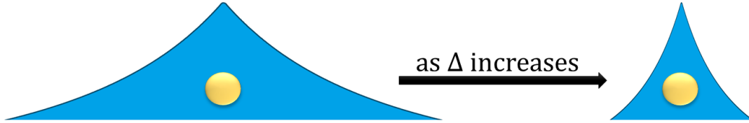
Figure 4.3: It reflects how the detuning change the photonic envelope around the atomic position and along with the effective cavity length.
