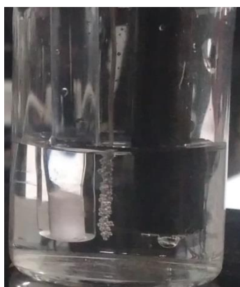
Figure A5.11: Evolution of hydrogen and oxygen bubbles at glassy carbon disk and Pt wire electrodes, respectively
