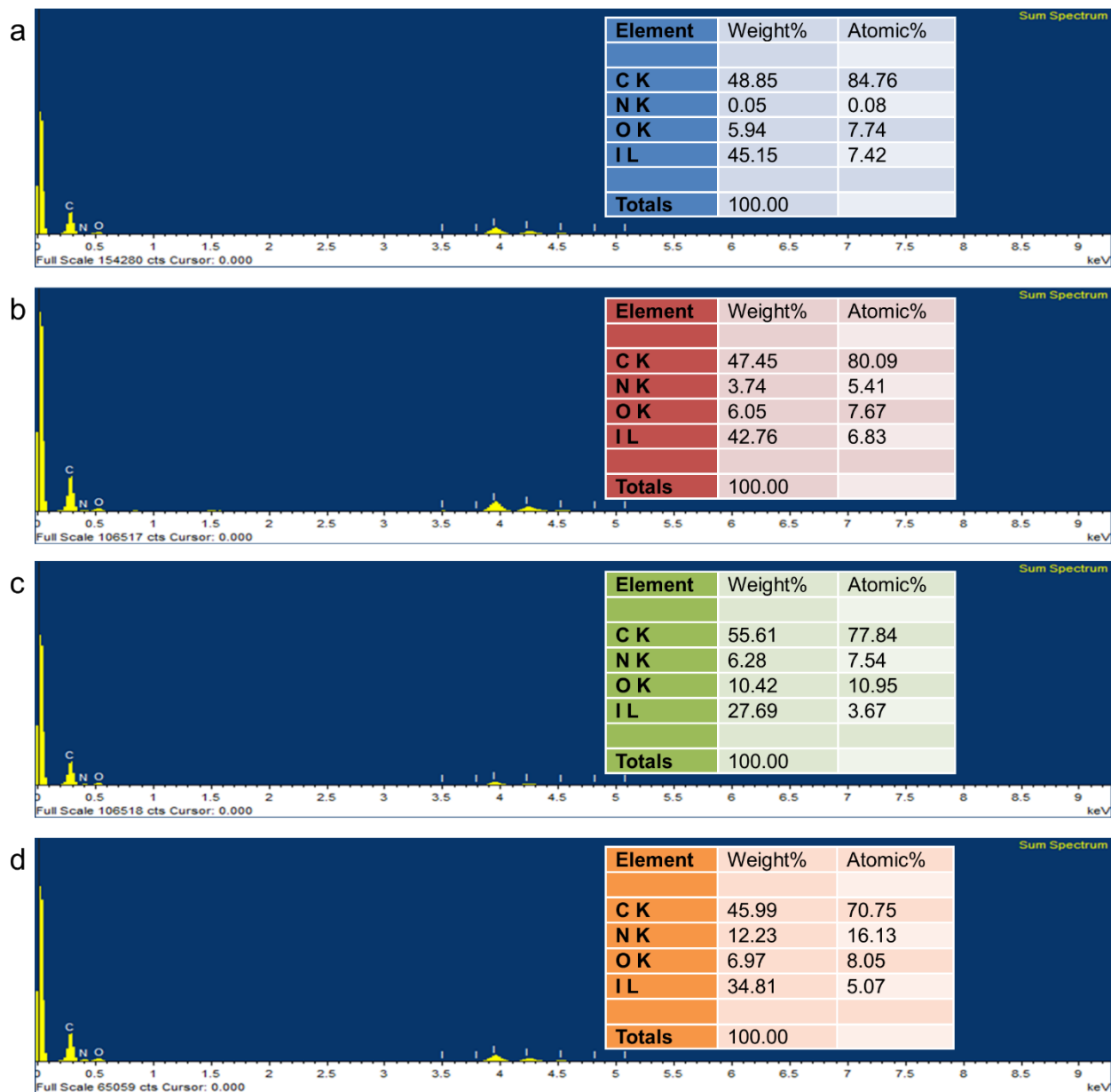
Appendix 2.30: Energy-dispersive X-ray spectroscopy (EDS) data from FESEM experiment of (a) CH 3 I@COF-A, (b) CH 3 I@COF-B, (c) CH 3 I@COF-C, and (d) CH 3 I@COF-D.
