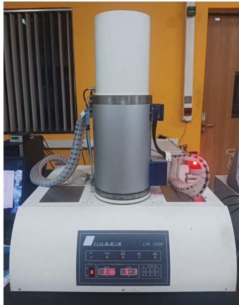
Figure 2.2.5: LFA-1000 setup for thermal diffusivity measurements
