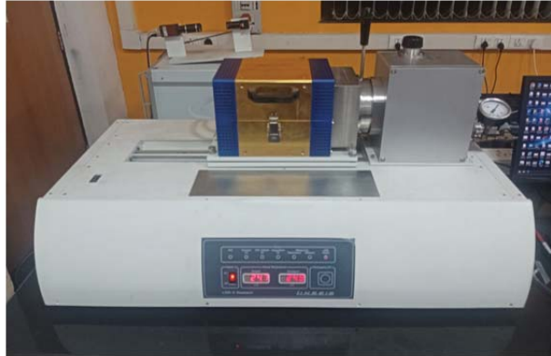
Figure 2.2.3: LSR-3 setup for Seebeck and resistivity measurements
