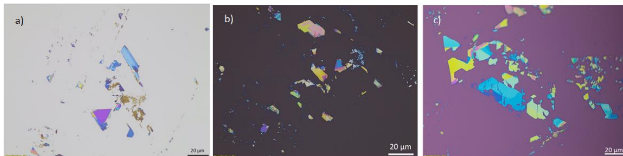
Figure 4.1: Exfoliated Sample of MnPS 3 on (a) pure Si substrate (b) 90nm SiO 2 /Si substrate (c) 285 nm SiO 2 /Si Substrate
