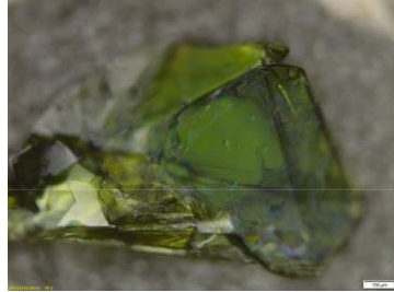
Figure 2.2: Bulk crystal of \text{MnPS}_3
