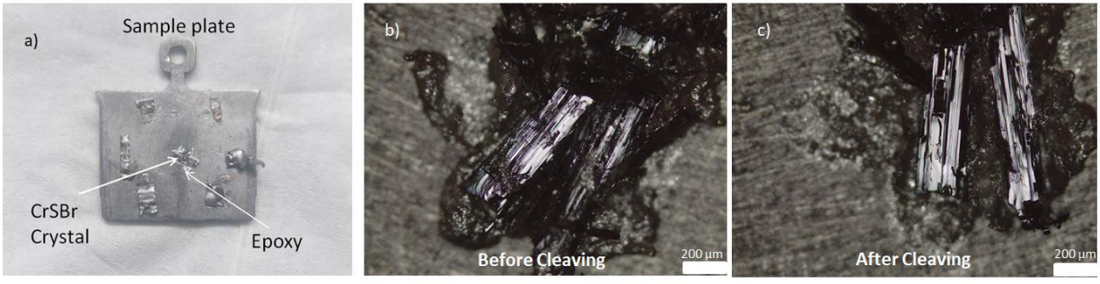
Figure 5.3: (a) Bulk Crystal on STM sample plate attached using silver epoxy, (b) Un-cleaved CrSBr crystal, (c) Cleaved CrSBr crystal.
