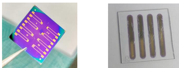
Figure 6. Optical images of the electrode configuration of two-probe and four-probe measurements
