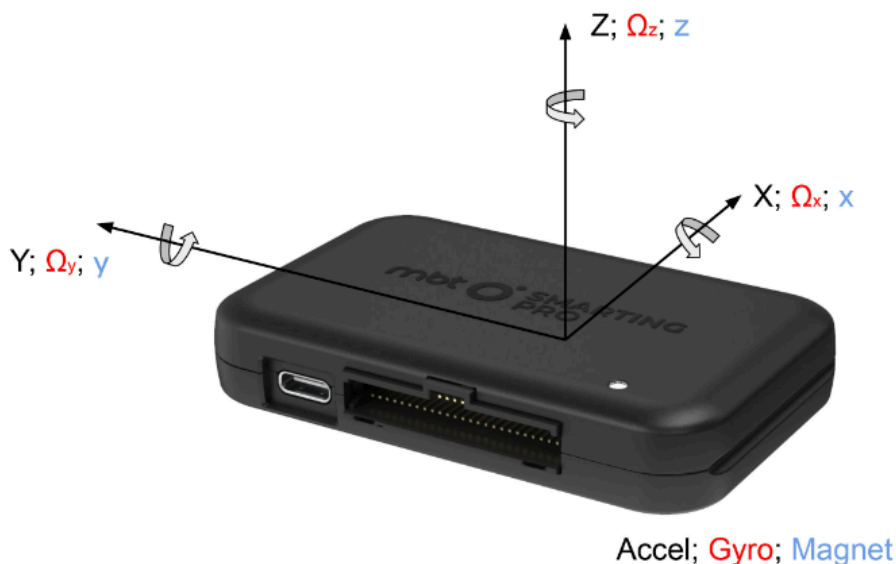
Fig 3.06 : The MBT Smarting Pro Device orientation. It has inbuilt IMU sensors (Accelerometer and Gyroscope) situated in the orientation provided below. It is placed in a upright orientation ( + X axis perpendicular to the ground) where subject's rotation is measured by rotation around X axis and forward motion is obtained from translation in z axis
