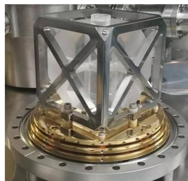
(d) 10cm Cubic cavity mounted on a bracket with tetrahedral symmetric support, built by NTSC, China [55].
