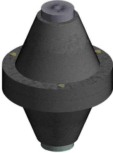
(a) Tetrahedral 3D mesh elements in cavity spacer and hexagonal mesh elements for mirrors & patches.
