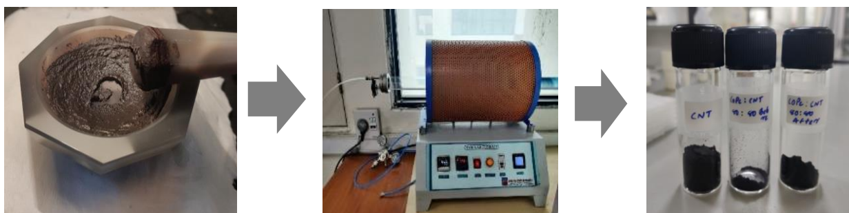
Figure 2.1: Steps involved in the pyrolysis of materials.
